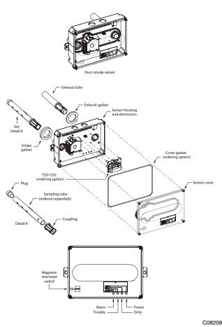
Fig. 17 - Smoke Detector Sensor
